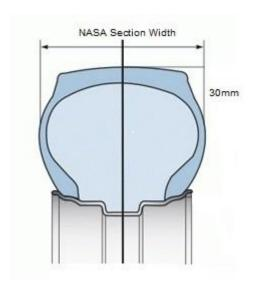
NASA Section Width tire measurement tools should be available at each NASA region technical inspection/impound area. The tool should fit loosely on the tire and not bind. It should fall if not being held in place. Additionally, templates for each tool size are available in a separate .pdf file on the NASA rules page.
