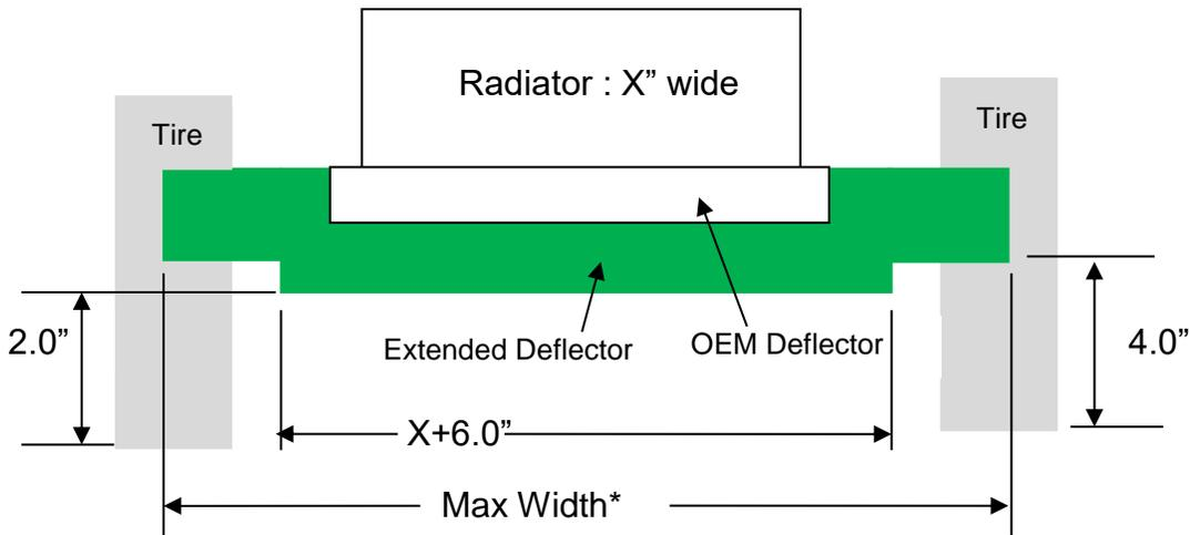
\* Max Width shall be 55" or the car's OEM air deflector, whichever is greater
