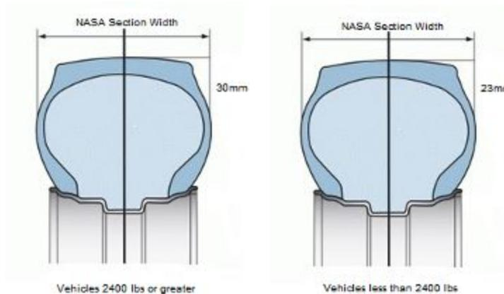
NASA Section Width tire measurement tools should be available at each NASA region technical inspection/impound area. The tool should fit loosely on the tire and not bind. It should fall if not being held in place. Additionally, templates for each tool size are available in a separate .pdf file on the NASA rules page.
