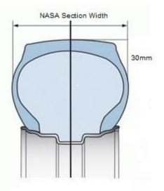
NASA Section Width tire measurement tools should be available at each NASA region technical inspection/impound area. The tool should fit loosely on the tire and not bind. It should fall if not being held in place. Additionally, templates for each tool size are available in a separate .pdf file on the NASA rules page.
